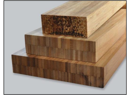
Figure 5: Laminated Bamboo Beams [8]
